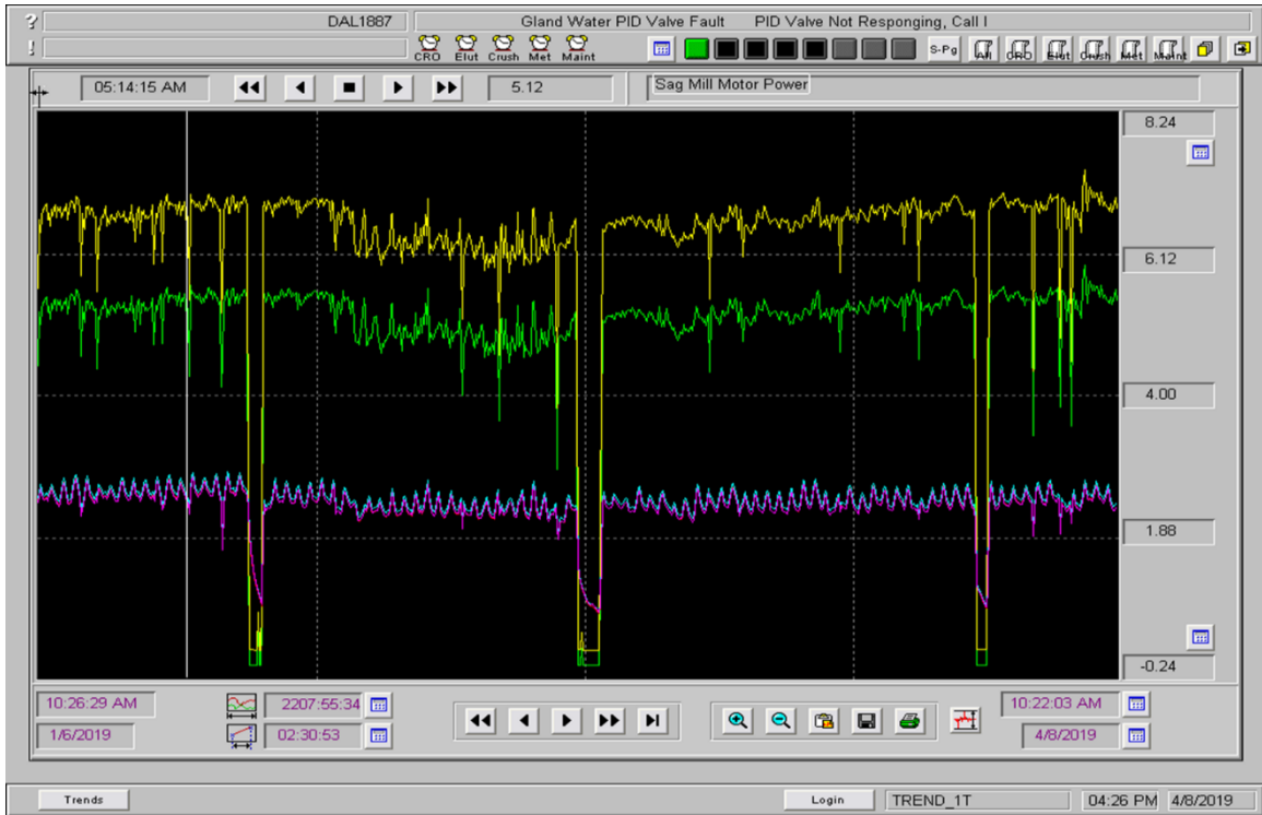
Fig. 4.3 Trends of SAG Mill Motor Current, Power and Winding Temperatures
