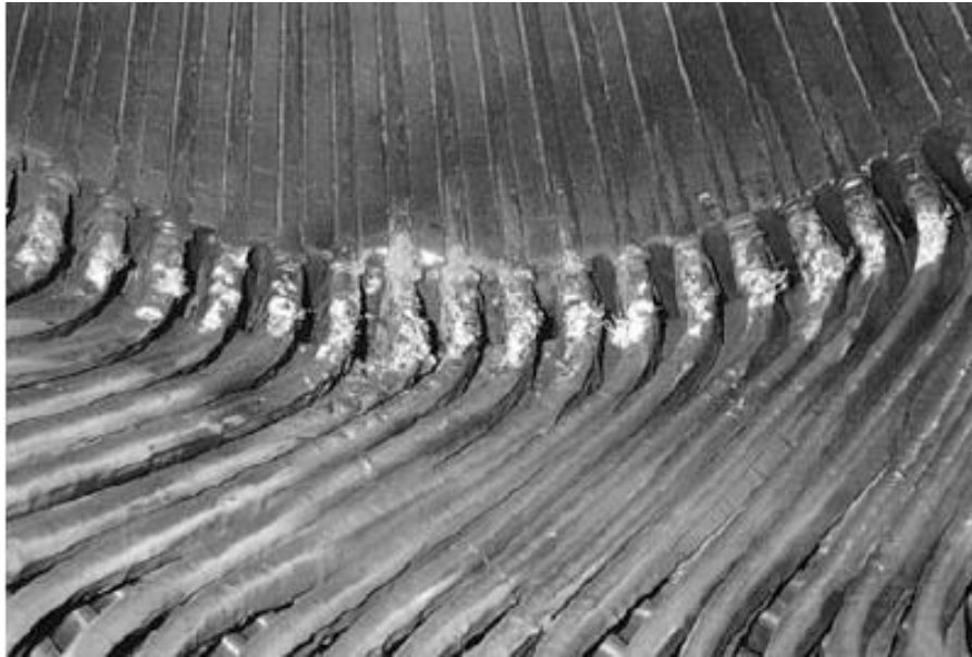
Fig. 2.26 Photograph of Damaged Stator Winding
