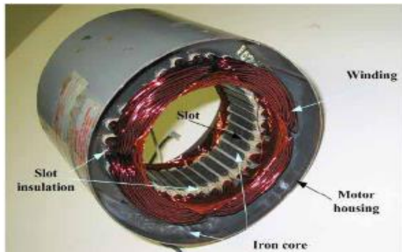
Fig. 2.2 Single Phase Stator with Windings
