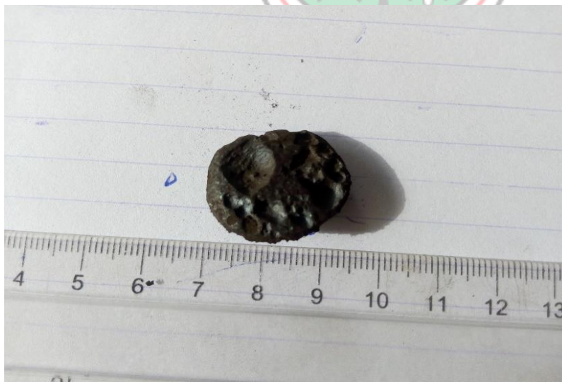
Figure 4.17: Reduced Metal Produced from Mbalam Iron Ore 1 Using ELT as Reducing Agent
