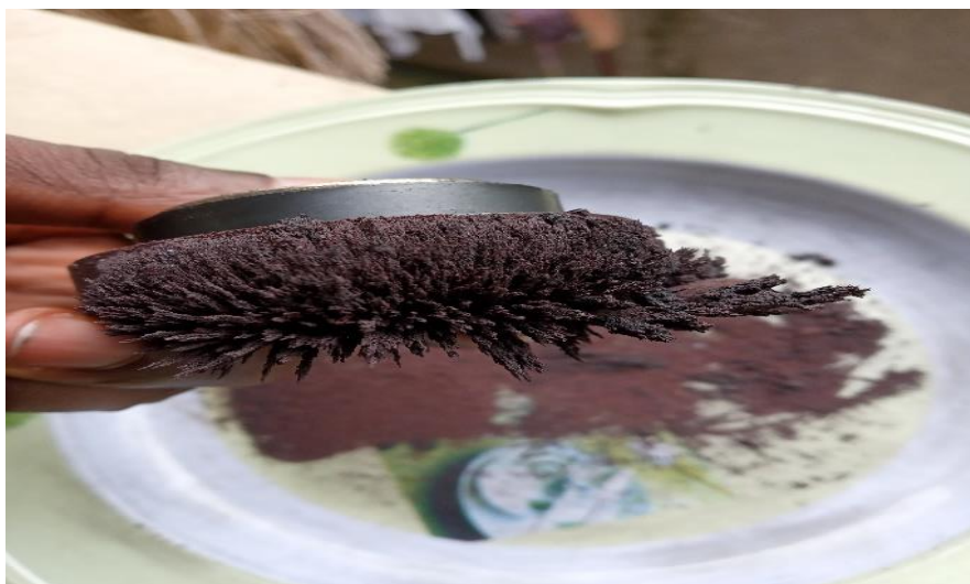
Figure 4.18: Reduced Metal Produced from Mbalam Iron Ore 3 Using PET as Reducing Agent.
