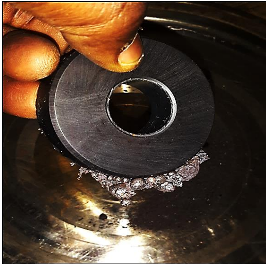
Figure 4.10 Reduce Metal Produced from Microwave Reduction held on a Magnet
