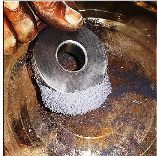
Figure 4.11 Reduce Metal Produced from 'Sika Bukyia' Reduction held on a Magnet
