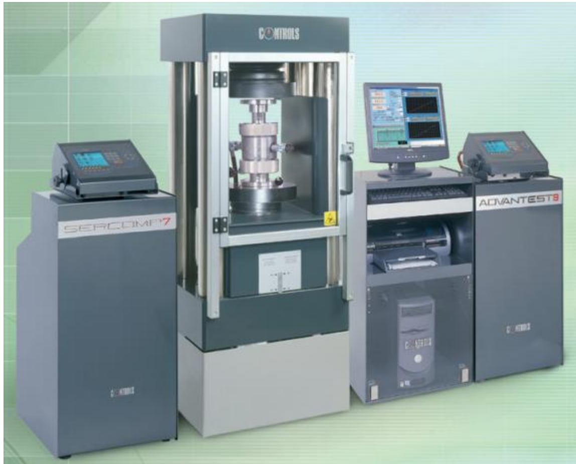
Figure: 4.6 The UCS Test Set-Up
