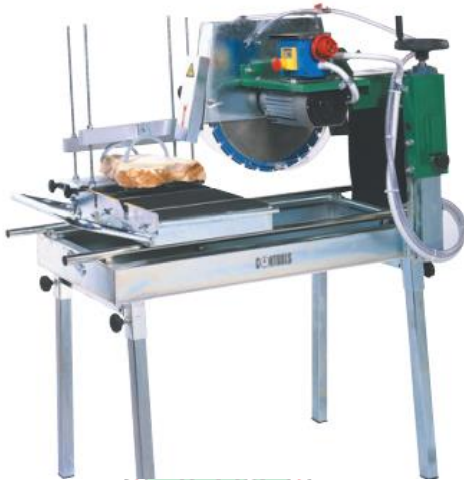
Figure 4.5 Rock Cutting Equipment Used for Laboratory Sample Preparation (Anon, 2017)
