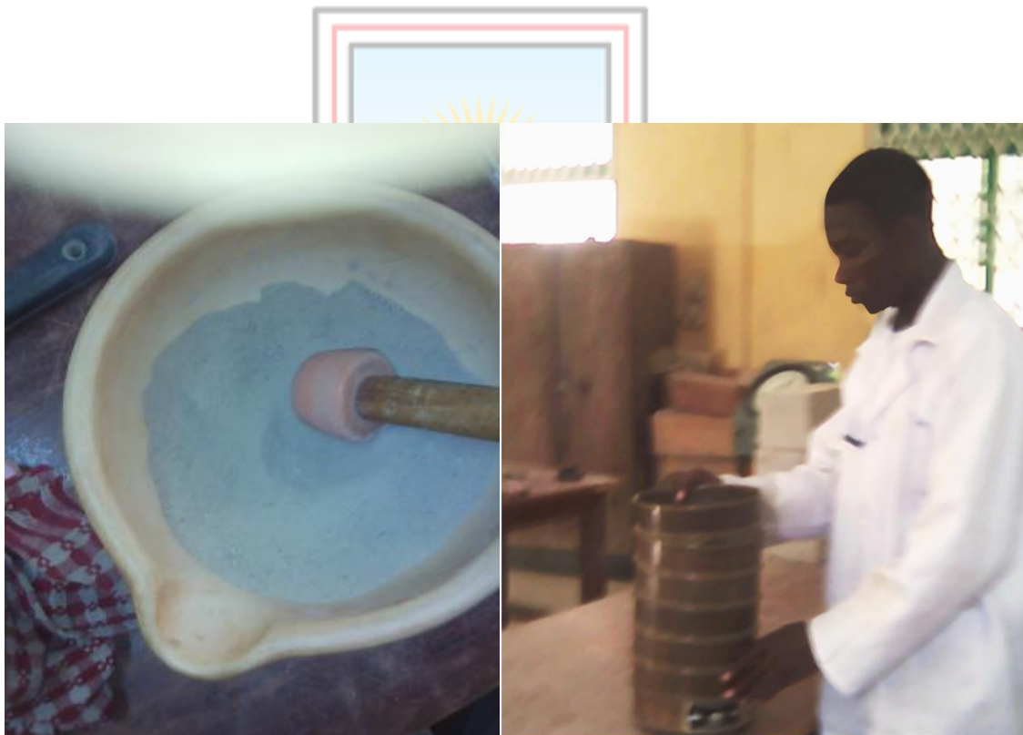
Figure 4.7 Sieving of Rock Aggregates
