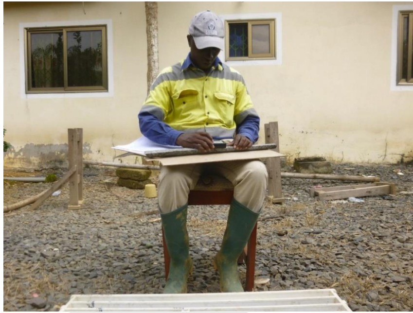
Figure 4.1 Magnetic Susceptibility Data Collection with SM-30
