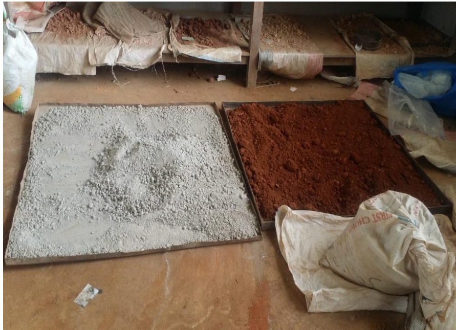
Figure 4.3 Air Drying of Samples
