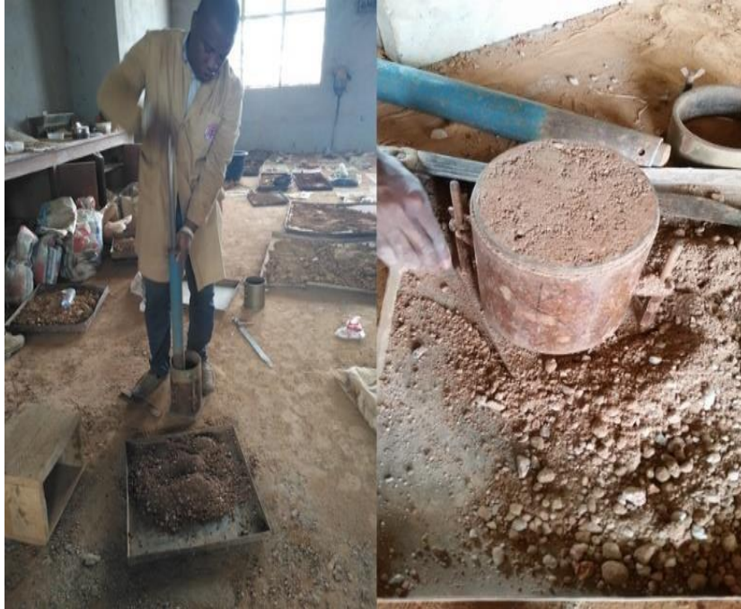
Figure 4.4 Compaction of Laterite and Spent
