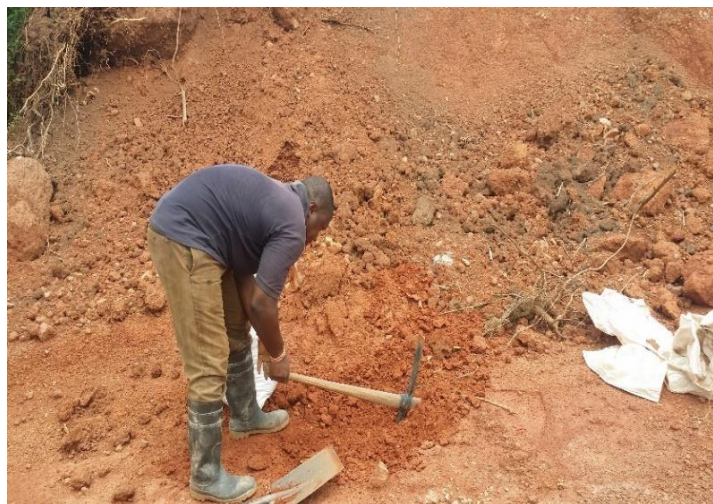
Figure 4.1 Excavation of Laterite Sample
