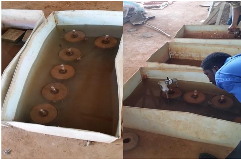
Figure 4.5 Soaking of CBR Samples and Measuring of Swell
