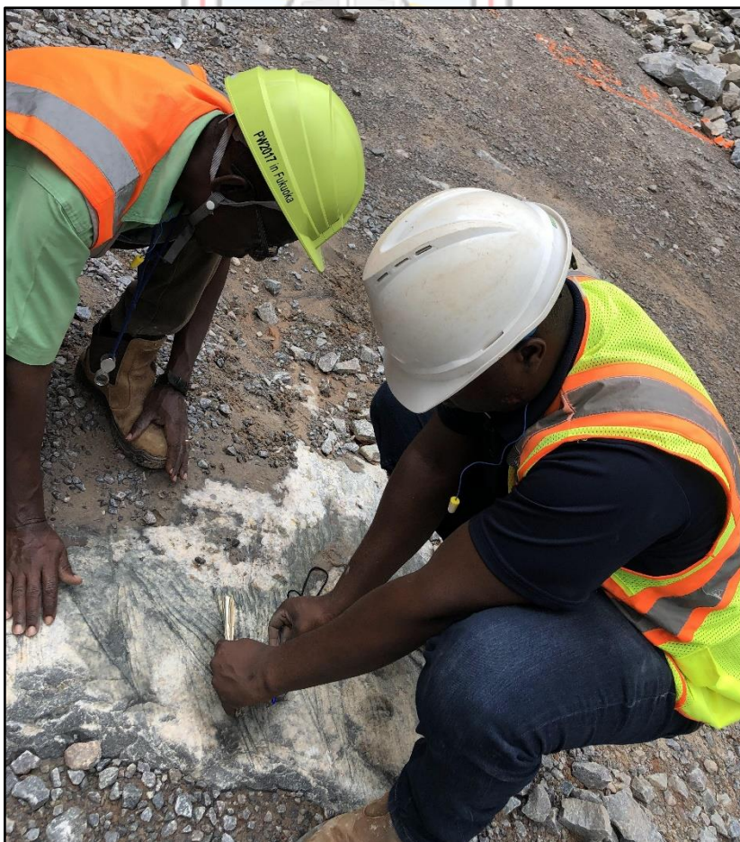
Fig. 3.1 Measurement of bedding and foliation in Banket Footwall Quartzite
