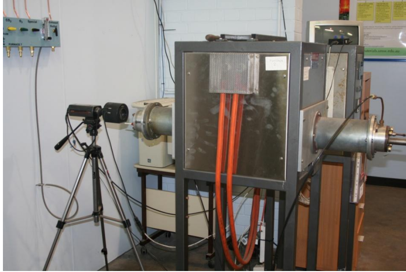
Fig. 3 Pictorial representation of the horizontal furnace
