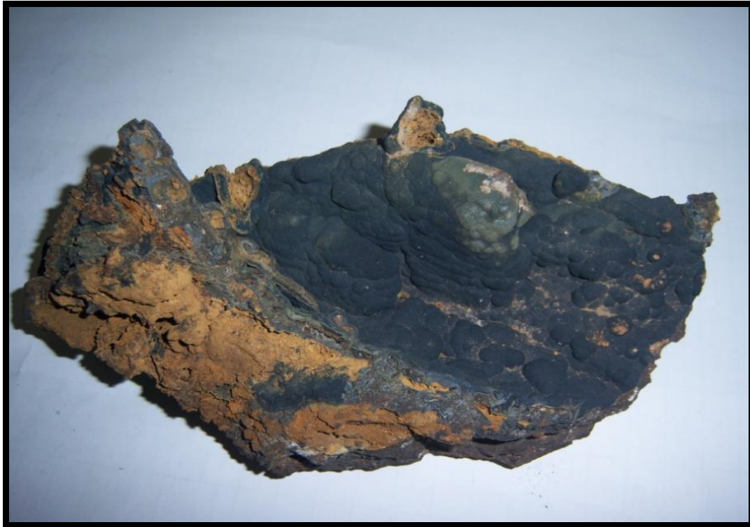
Fig. 6 High grade manganese oxide ore, commonly known as Nsutite, which has been mined in Nsuta since 1914
