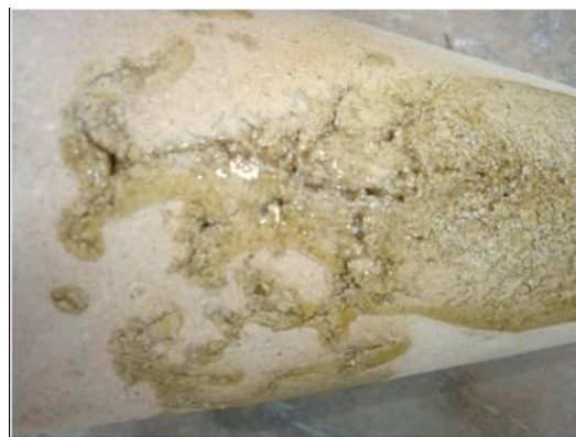
Fig. 11 Molten charge that has seeped out of a crucible during fusion
