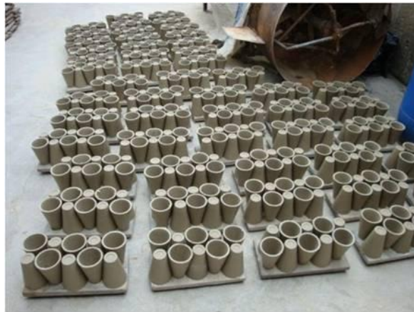
Fig.5 Moulded crucibles being dried in the open
