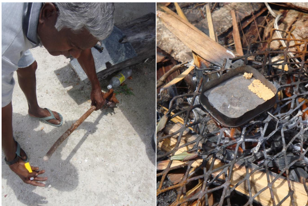
Left: Metal retort. Right: Open burning of amalgam on fire
