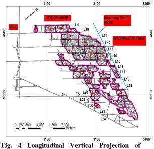
Fig. 4 Longitudinal Vertical Projection of Stoped-out Areas in the WL-WR Compartment of the AVS.
