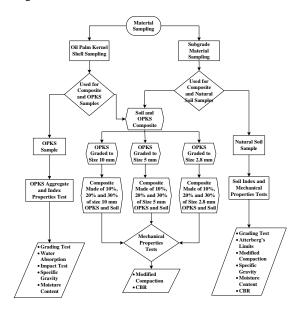
Fig.1 Flow Chart of Test Methods and Materials
