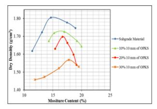
Fig.6b Modified Compaction Curves of Natural Soil and 10 mm OPKS
