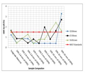
Fig. 8 CBR Swell of Natural Soil and Composite Materials
