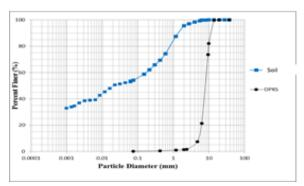
Fig.5 Grading Curves of Natural Soil and OPKS
