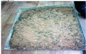
Fig. 4 Composite of a Graded OPKS and Natural Soil
