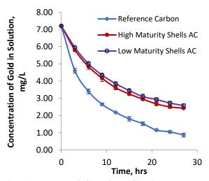
Fig. 1 Recovery of Gold from Solution by the Activated Carbons obtained after 1 hr Activation and the Reference Activated Carbon
