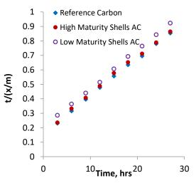
Fig 6 Adsorption Rate of ACs obtained after 3 Hours Activation
