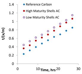
Fig. 5 Adsorption Rate of ACs Obtain after 2 Hours Activation
