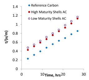
Fig 4 Adsorption Rate of ACs obtained after 1 Hour Activation
