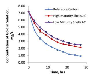
Fig. 2 Recovery of Gold from Solution by the Activated Carbons obtained after 2 hrs Activation and the Reference Activated Carbon
