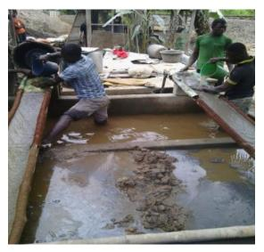
Fig. 1 Gravity Concentration by Sluicing
