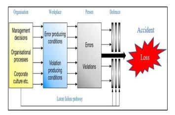
Fig. 3 SCM Mark II Adapted (Reason et al., 2006)
