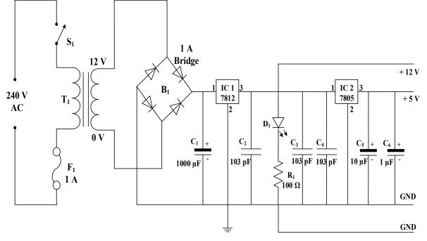
Fig. 2 12 V and 5 V Power Supply Circuit
