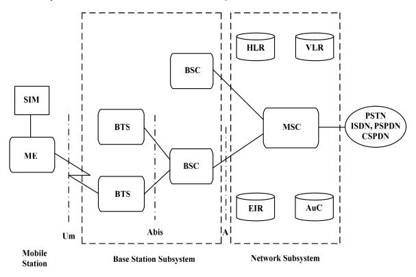
Fig. 6 General Architecture of a GSM Network
