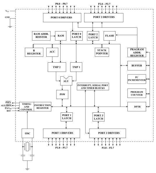
Fig. 3 Architecture of AT89C51 Microcontroller
