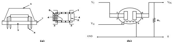
Fig. 4 (a) Structure of the MQ-5 Gas Sensor and (b) Basic Measuring Circuit of MQ-5 Gas Sensor
