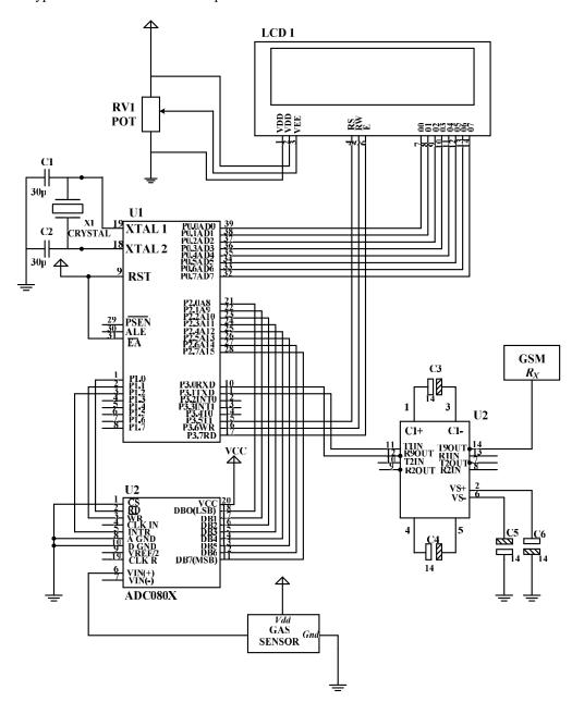
Fig. 9 Circuit Diagram of the Proposed System
