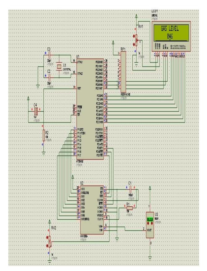
Fig. 10 Simulation Model of the LPG Leakage Detector
