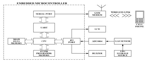
Fig. 7 Design Concept Diagram of the Proposed System
