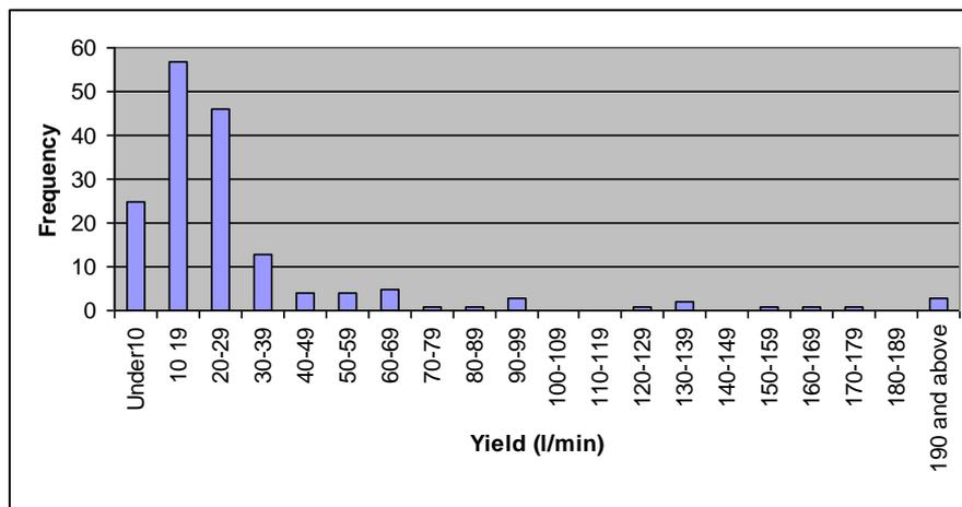
**Fig. 3 Graph of Boreholes Yield versus Frequency**
