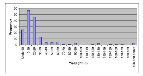
Fig. 3 Graph of Boreholes Yield versus Frequency
