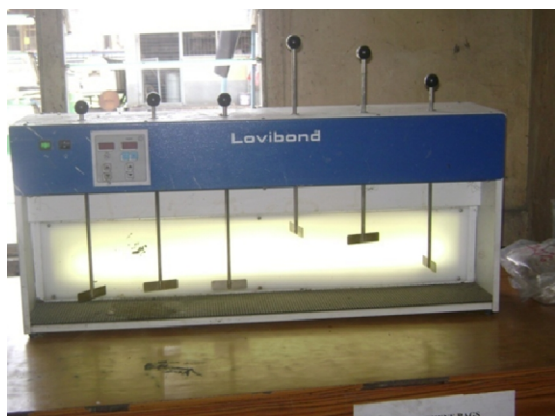
Fig 1 Six-stirrer Lovibond Flocculator
