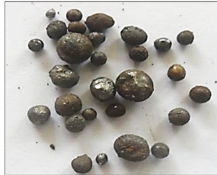
Fig. 7 Spherical Particles of Metallic Iron Produced after Reduction
