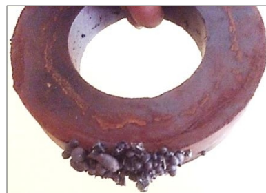
Fig. 8 Attraction of Metallic Spheres to a Low Intensity Magnet
