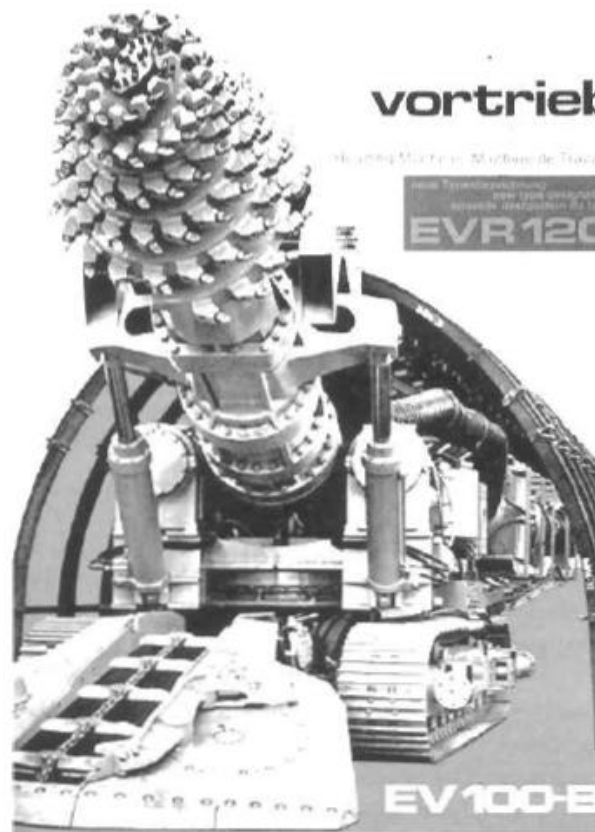
Fig. 12. The roadheader machine (from Sugden, 2005).
