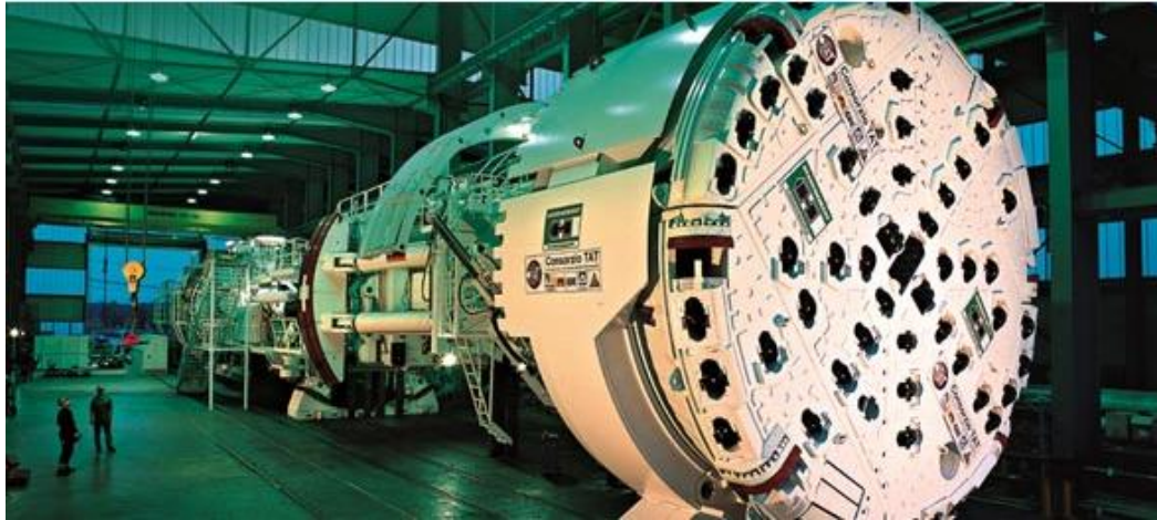
Fig. 13. Typical Gripper TBM for hard rock tunneling.
