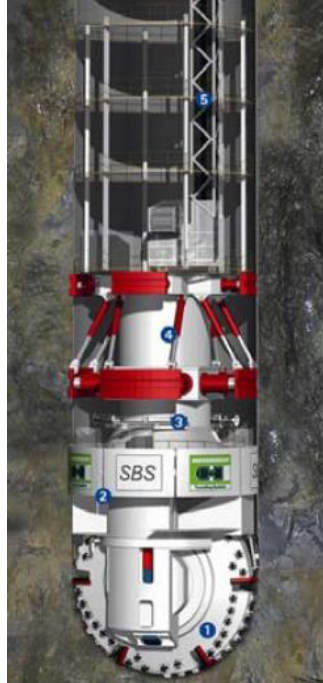
Fig. 18. Shaft boring system (SBS) for sinking shafts in hard rocks, up to 2000 m-depth (from Frenzel et al., 2010).
