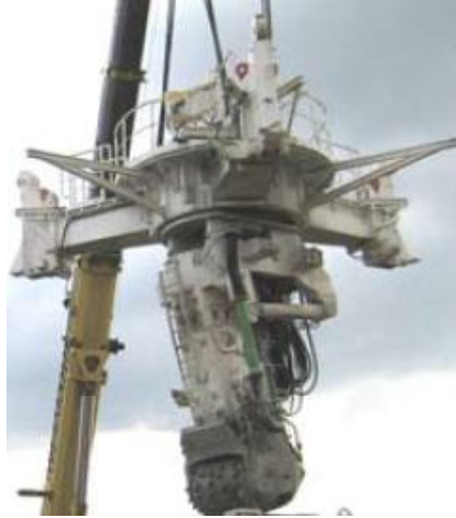
Fig. 14. Adaption of the roadheader for shaft boring (from Frenzel et al., 2010).
