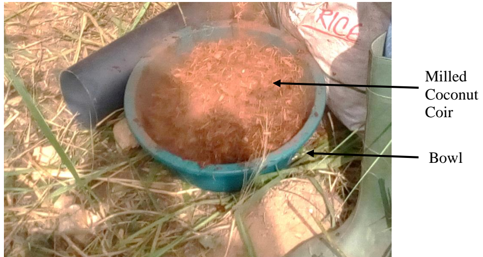
Figure 3.5 Coconut Coir Ready to be backfilled
