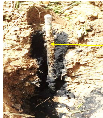
Figure 5.5 A rod Buried with Tyre Ash
