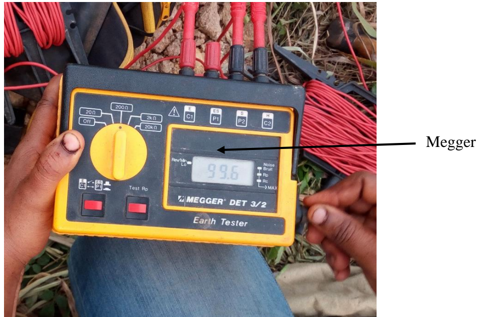
Figure 3.13 Megger Showing Resistance Value
