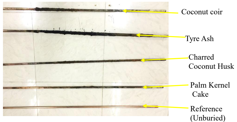
Figure 5.6 Rods Removed from the Soil
