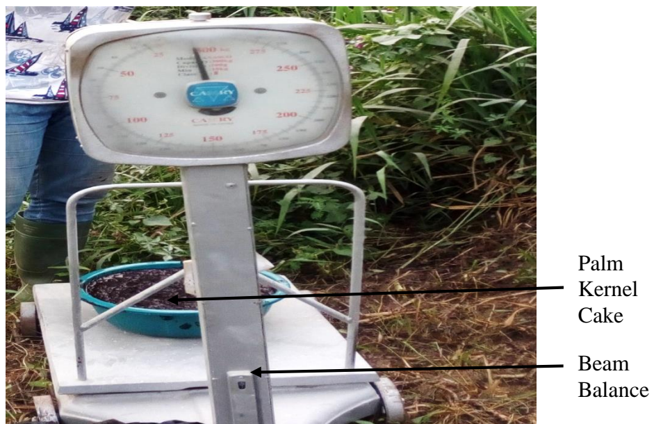
Figure 3.14 Backfill Material being Weighed
