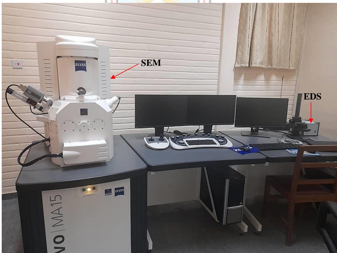
Figure 2.4 Scanning Electron Microscope (SEM) Equipped With An Energy Dispersive X-Ray Spectrometer (EDS)
