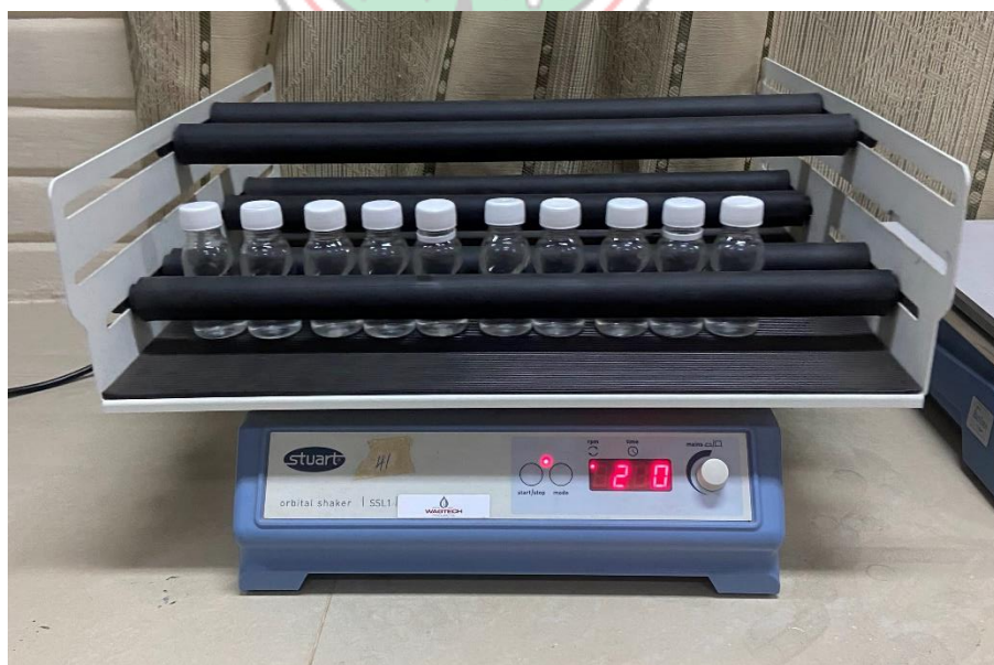
Figure 3.6 AgNP-PVA/NRL Nanofibre Composites in Hg Solution Agitated on an Orbital Shaker
