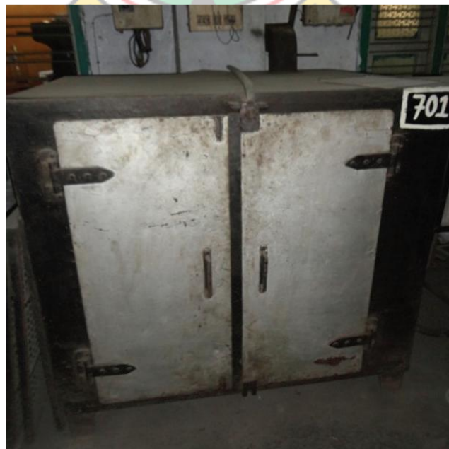
Figure 2.24 A Typical Post Curing Furnace (Source: Suryarajan et al. , 2016)
