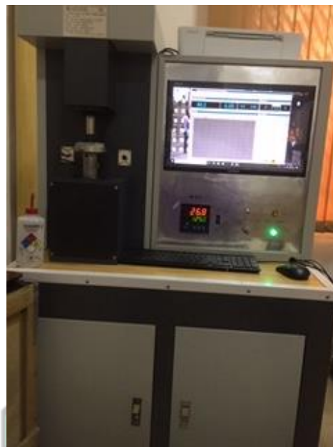
Figure 3.26 Setup of the Universal Friction and Wear Testing Machine
