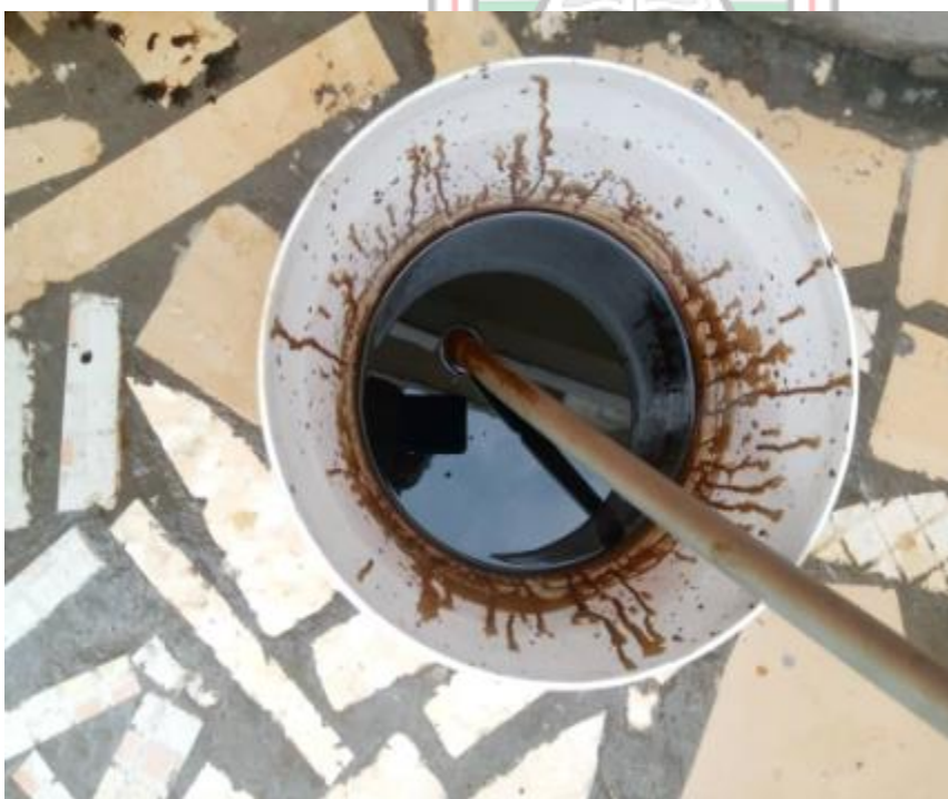
Figure 3.23 The mixture of the hot water and crude oil stirred in a basin
