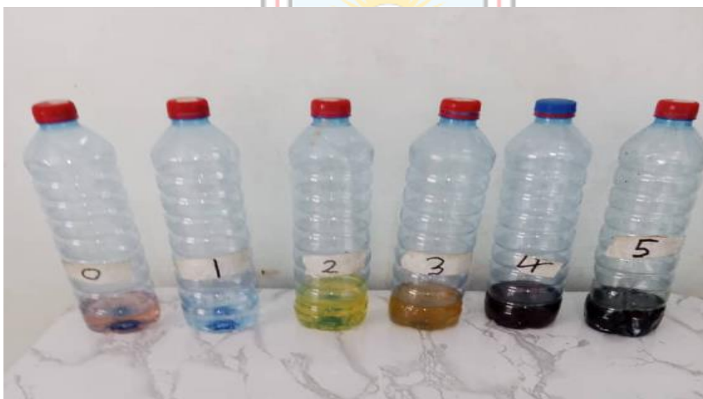
Figure 3.45 Crude Oil Fractions (Sample 0, Gasoline; Sample 1, Naphtha; Sample 2, Kerosene, Sample 3, Diesel, Sample 4, Fuel Oil; Sample 5, Bitumen)
